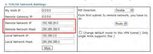
Please check if the VPN connection is built successfully in both devices respectively. For Vigor3900, open VPN and Remote Access>>IPSec>>Status for viewing the result.
