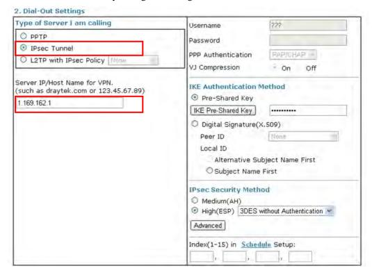
3. For the role of Vigor2710 is dialing-out, please skip Dial-In setting. Type the **Remote Network IP** and **Remote Network Mask** of Vigor3900 to complete configuration.
