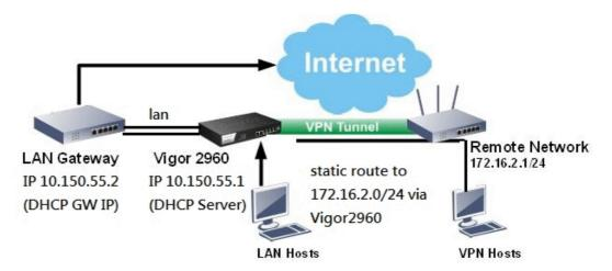
1. Go to **LAN** >> **General Setup** >> lan1 click **Edit**, input the Gateway IP you'd like to assign to DHCP clients in **DHCP Routers** field and then **Apply** it.
