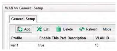
5. Create a new WAN profile named with **wan1\_1**, and set VLAN ID named with **111** based on WAN Port 1(WAN1). Note that **Untag** must be set with **Disable**. It means wan1\_1 can accept the packets tagged with VLAN ID 111. Next, click **Apply** to save the settings.
