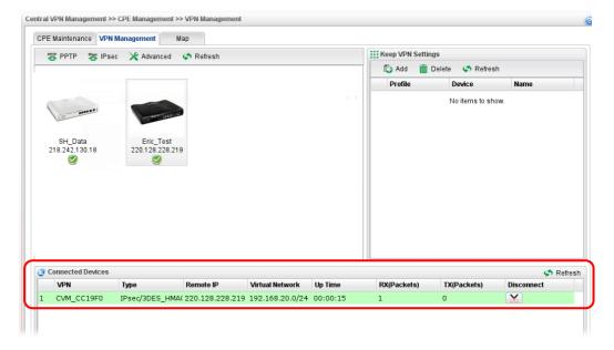
6. A LAN to LAN profile for such VPN will be generated automatically. You can access into **VPN and Remote Access>>LAN to LAN** of the remote device for viewing the detailed information.
