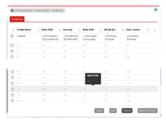
Check the box on the left side of the selected profile to modify the content of the profile. The **Clone**, **Edit** and **Apply To Device** buttons will be available then.
