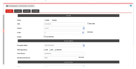
5. When you finished the above web page configuration, click **Finish** to exit and return to the first page. The modified WLAN profile will be shown on the web page.
