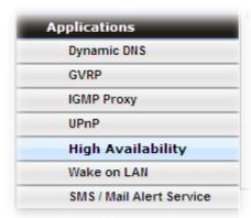
3. In the tab of **High Availability Global Setup**, choose **Hot-Standby** as Redundant Method; choose **Secondary** as Config Synchronization Rule; type the lan1 IP address configured in router A; type **draytek** as Authentication Key; choose **Automatic** as Advance Preemption Mode. Click **Apply** to save the settings.
