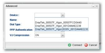
Specify the CPE from the Device drop down list; choose the name of the CPE; select PPTP or IPsec as the Dial Type; choose PAP\_only or PAP\_or\_CHAP as PPP authentication; enable or disable VJ Compression; then click **Connect** to build the VPN connection.
