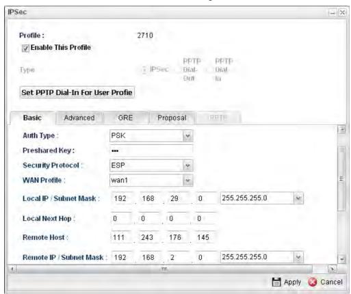
Type the Pre-shared key and choose a WAN Profile. Specify Local IP/Subnet Mask with 192.168.29.0/24. The Remote Host should be Vigor 2710's WAN IP address; and the Remote IP/Subnet Mask should be 192.168.2.0/24.
