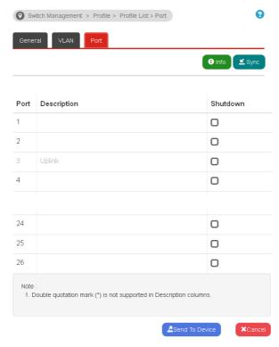
After finished the port configuration, click the VLAN tab to modify settings relevant to VLAN.
