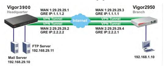
Vigor3900 allows users to build VPN load balance connection between Vigor3900 and other router. Take Vigor2950 for an example. There are two WANs on Vigor2950 and two WANs on Vigor3900. We will build VPN connection with load balance between Vigor3900 and two WANs of Vigor2950 respectively.
