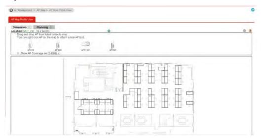
4. Check the box of **Show AP Coverage on** 5GHz/2.4 to display the signal coverage area.
