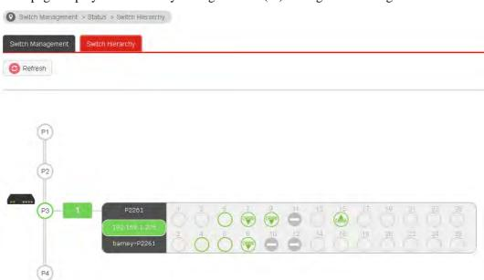
**Note**: If the hierarchy display is incorrect, please access into the web user interface of VigorSwitch and enable the function of LLDP (e.g., Configuration >>DDLP>>LLDP General Setup in VigorSwitch 2261). The interval for LLDP shall be less than 3 minutes (the default setting, 30 seconds).
