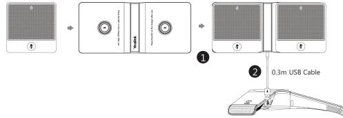
During charging, the battery LED indicator on the CPW90 glows solid red. When the battery capacity reaches 100%, the battery LED indicator on the CPW90 will glow solid green.
